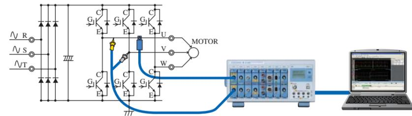
Line voltage is measured by 100MS/s 12-bit isolation module and 10MS/s 12-bit isolation module. Limited time resolution at 10MS/s (yellow line). High time resolution at 100MS/s (red line).
