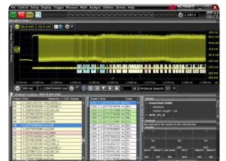
Trigger on and decode MIPI packets
