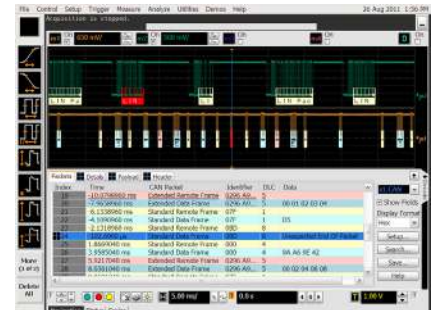
Trigger on and decode CAN, LIN and FlexRay serial packets.
