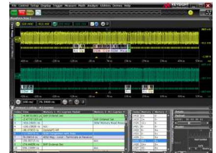
Trigger on and decode PCIe serial packets.
