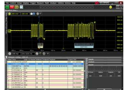
Trigger on and decode USB packets.
