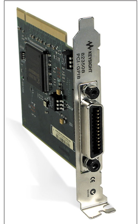
82350B PCI high-performance GPIB interface card
