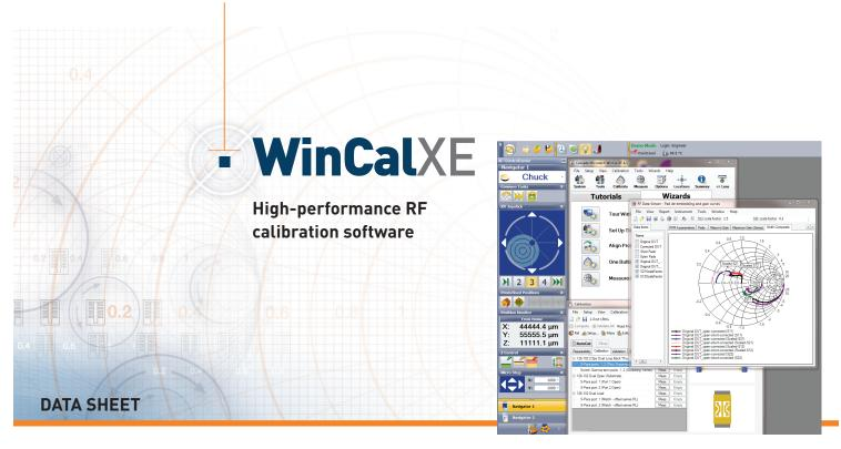
Cascade Microtech's WinCalXE™ software is a comprehensive and intuitive on-wafer RF measurement calibration tool to achieve accurate and repeatable S-parameter measurement, which is crucial for precision device modeling/characterization and engineering RFIC test.
