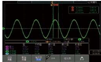
IT7600 after paralleling of 3 sets, each unit will share the test current averagely
