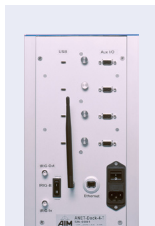
Rear View of the ADock Tower Variant
