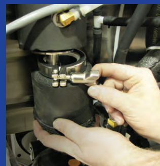
Steam generator removes for easy cleaning
