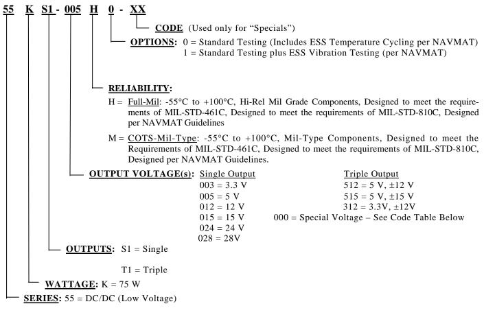
*Example:* 55KS1-005H0 = DC/DC (Low Voltage); 75 Watt; Single Output; +5 V; Full-Mil-Type; Standard Testing 55KD1-012M1 = DC/DC (Low Voltage); 75 Watt; Dual Output; ±12 V; COTS-Mil-Type; ESS Vibration Testing 55KT1-515M1 = DC/DC (Low Voltage); 75 Watt; Triple Output; 5 V, ±15 V; COTS-Mil-Type; ESS Vibration Testing
