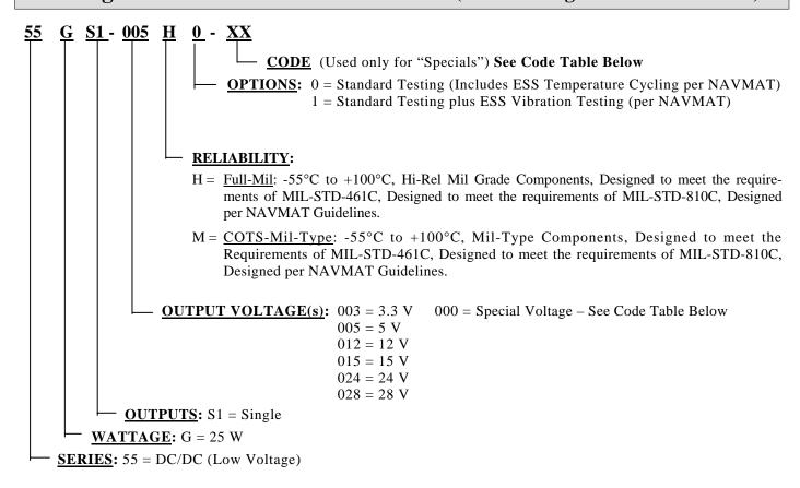
**Example**: 55GS1-005H1 = DC/DC (Low Voltage); 25 Watt; Single Output; +5 V; Full-Mil-Type; ESS Vibration Testing 55GS1-012M0 = DC/DC (Low Voltage); 25 Watt; Single Output; +12 V; COTS-Mil-Type; Standard Testing
