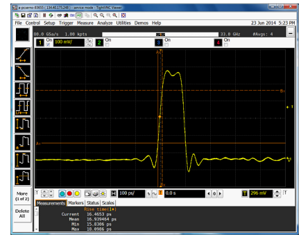
Figure 5. 100 ps pulse with 17 ps risetime.
