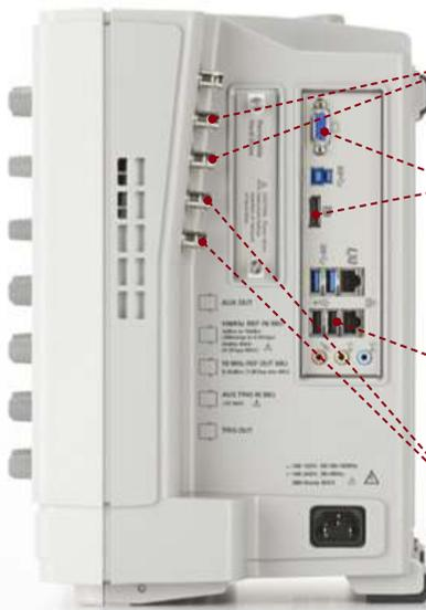
Built-in 10-MHz reference in/out ports synchronizes multiple measurement instruments in a system
