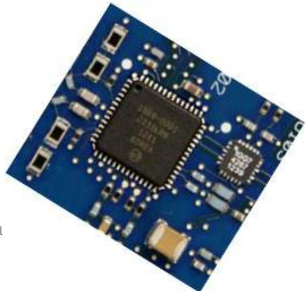
S-Series front-end includes three new custom ICs including a 130 nm BiCMOS IC that incorporates user-selectable analog filters and bandwidth upgrades via a software license.
