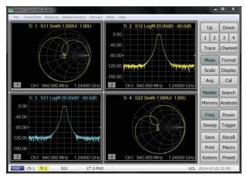
The PXI VNA interface guides test engineers using a similar look and feel as Keysight's popular PNA family of network analyzers.
