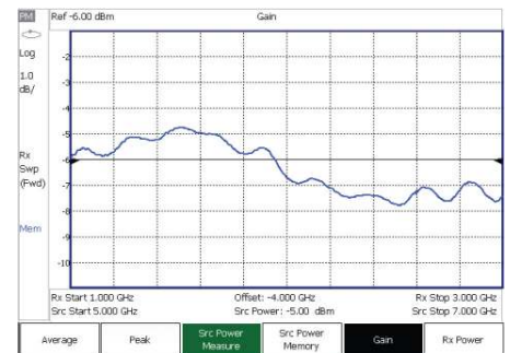
Characterize mixers with FieldFox and a USB power sensor
