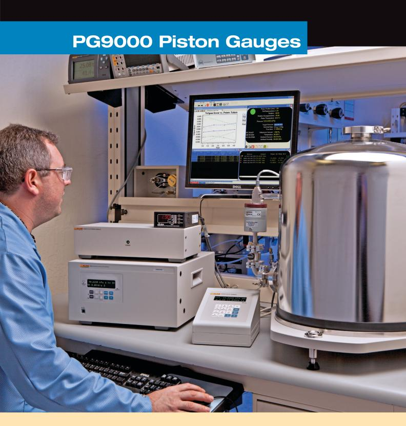
Automated primary pressure reference for absolute and gauge pressures to 10 MPa
