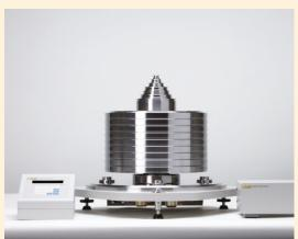
PG9000 piston gauges are the next generation of absolute pressure piston gauges from Fluke Calibration. They are designed to enable metrology and research institutes to realize and disseminate exceptional fundamental pressure measurements. Each PG9000 model supports the use of up to a 100 kg mass load in absolute and gauge pressure operation, creating a wide usable pressure range for each piston-cylinder and enabling more overlap of ranges for intercomparison.
