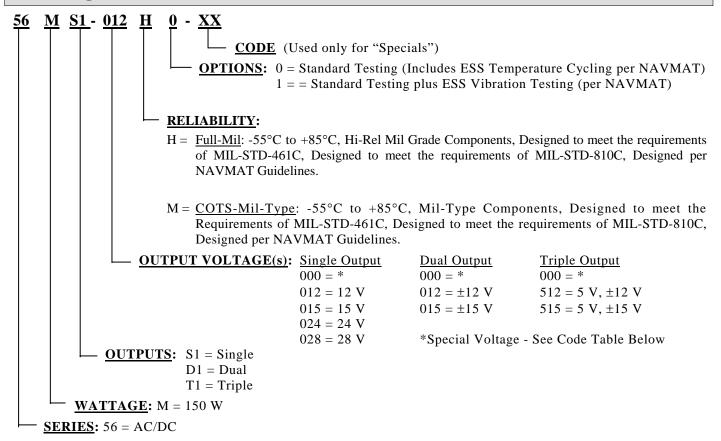
**Example:** 56MS1-012H0 = AC/DC; 150 Watt; Single Output; +12 V; Full-Mil-Type; Standard Testing 56MD1-012M1 = AC/DC; 150 Watt; Dual Output; ±12 V; COTS-Mil-Type; ESS Vibration Testing
