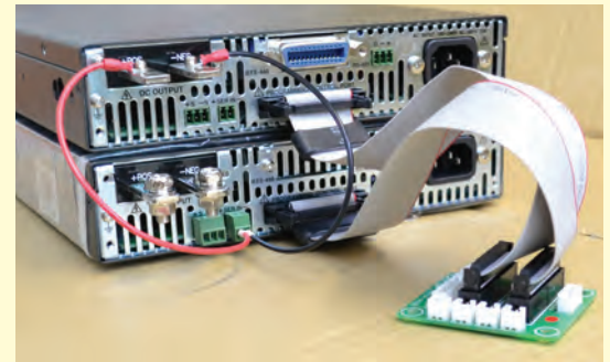
Series connection of two identical KLN power supplies using optional Series Socket Board 536-0130 and Programming Port Cable 518-0119
