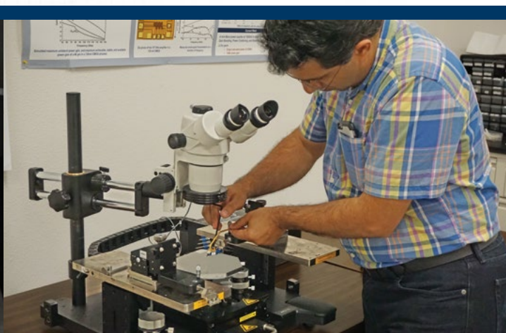
Dr. Momeni installing the Infinity Probe on his EPS150RF probe system.
