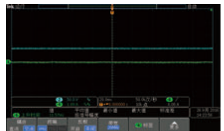
CV 50V high speed mode: CV stability, no vibration phenomenon
