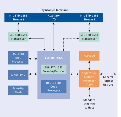
Per default, the ASP executes the AIM Network Sever (ANS) for use by customer applications via the Standard AIM Application Programming Interface. ASP Application Software development is supported via the Standard Ethernet Interface. A cross tool chain for ASP can be provided and also standard Linux debugging features like GDB are available. The use of onboard processing and large memory enables autonomous operation with minimal interaction with the host PC.
