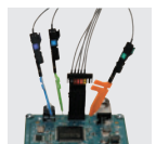
Example of logic probe connection
