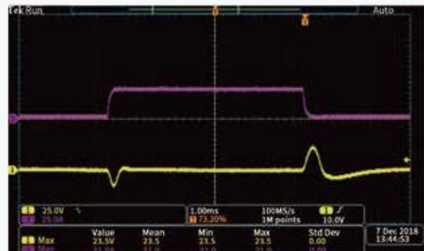
IT6006D-500-40 500V/40A/6kW Setting: voltage 100V current 28A Load current: 30A
