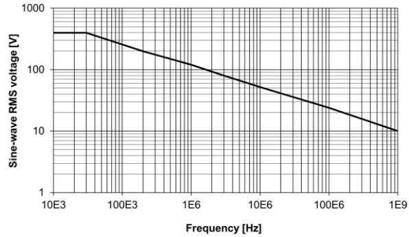
*R&S<sup>®</sup>RT-ZP03 maximum rated sine-wave root mean square voltage versus frequency (CAT I)*
