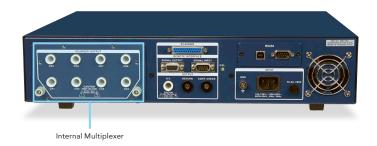
The HypotULTRA® models 7820 and 7850 offer a 4 or 8 channel HV internal scanner as an option. Additionally, the OMNIA® II models 8204 and 8254 offer an 8 channel HV and 8 channel HC internal scanner option. The high voltage channels can be configured from the front panel of the instrument or through Autoware®3. This model is perfect for cable harness and motor manufacturers that must subject multiple test points to high AC or DC voltages.
