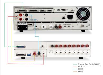
An OMNIA® II or HypotULTRA® electrical safety testing instrument and external SC6540 multiplexer are an ideal solution for appliance or medical device manufacturers that must perform multiple safety tests at different points on each product. The SC6540 multiplexer can be configured from the front panel of the test instrument or through Autoware®3.
