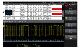
The 1000 X-Series is a powerful protocol analyzer that enables hardware-based specialized serial communication analysis (standard). Other vendors' oscilloscopes use software post-processing techniques that slow down the waveform and decode update rate, but the 1000 X-Series has faster decoding based on hardware technology that enhances scope usability and the probability of capturing infrequent serial communication errors.
