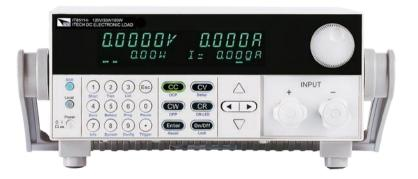
IT8500+ series single channel programmable electronic load with high density, high resolution and high accuracy supports dynamic test function, automatic test function, etc., which is suited for applications in areas such as LED driver testing, switching power testing, battery performance testing, etc. IT8500+ also provides standard SCPI protocol to build intelligent test platform that is ideal for multiple industries.
