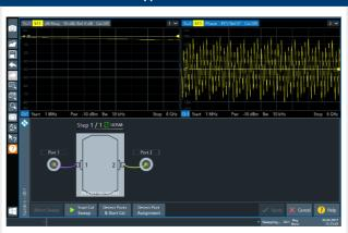
Automatic calibration units supported for convenient automatic system error correction. To be even quicker, a one-step auto cal is available.
