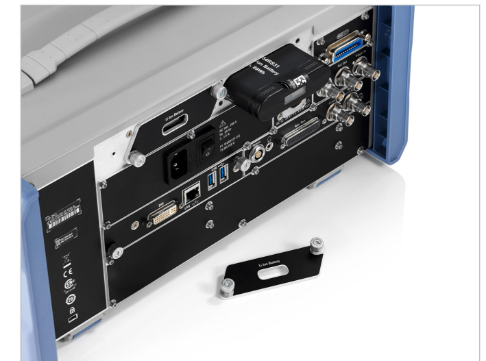
Rear view of the R&S®ZNL with battery compartment. The batteries can be easily accessed.
