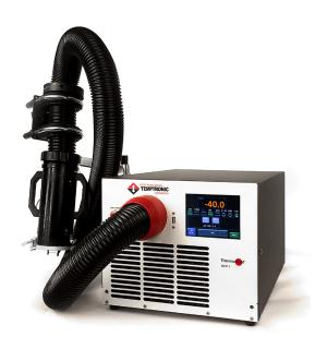
User-programmable temperatures, graphing, and data logging are established through the controller's touch-screen or remote communications. The system provides fast and precise transitions of temperature at the IC, even with variations in device power, and can be used with Temptronic's proven DUT Control technology using an imbedded diode or external thermocouple.
