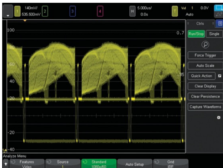
Figure 27. Triggering on 1080p HDTV signal analysis.
