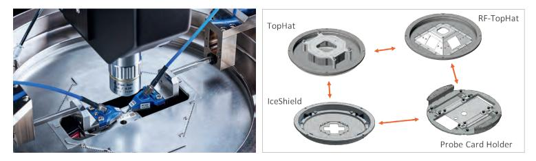
IceShield<sup>™</sup> is an optional platen insert that can be used as an open alternative to the TopHat. It enables frost-free operation down to -60°C<sup>1</sup> in an open environment. It is ideal for applications that require short cable lengths, such as S-parameter and load-pull measurements, and do not require EMI shielding or a dark measurement environment.
