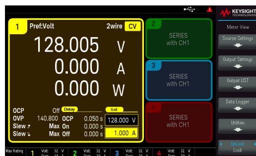
Figure 3: Increase output voltage with E364SNP kit.
