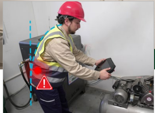
Traditional acoustic imager operation
