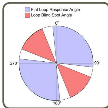
It was chosen to orient this blind spot at 45° and further to rotate every other row by 90° so that consecutive rows do not have the same blind spots. Because of this arrangement the blind spot can be eliminated by measuring a DUT twice with a small physical shift between scans.
