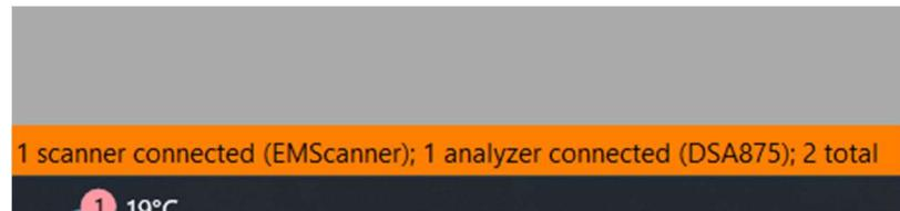
The **EMViewer** software automatically searches for devices. If a device is not connected properly, **EMViewer** will not display it.
