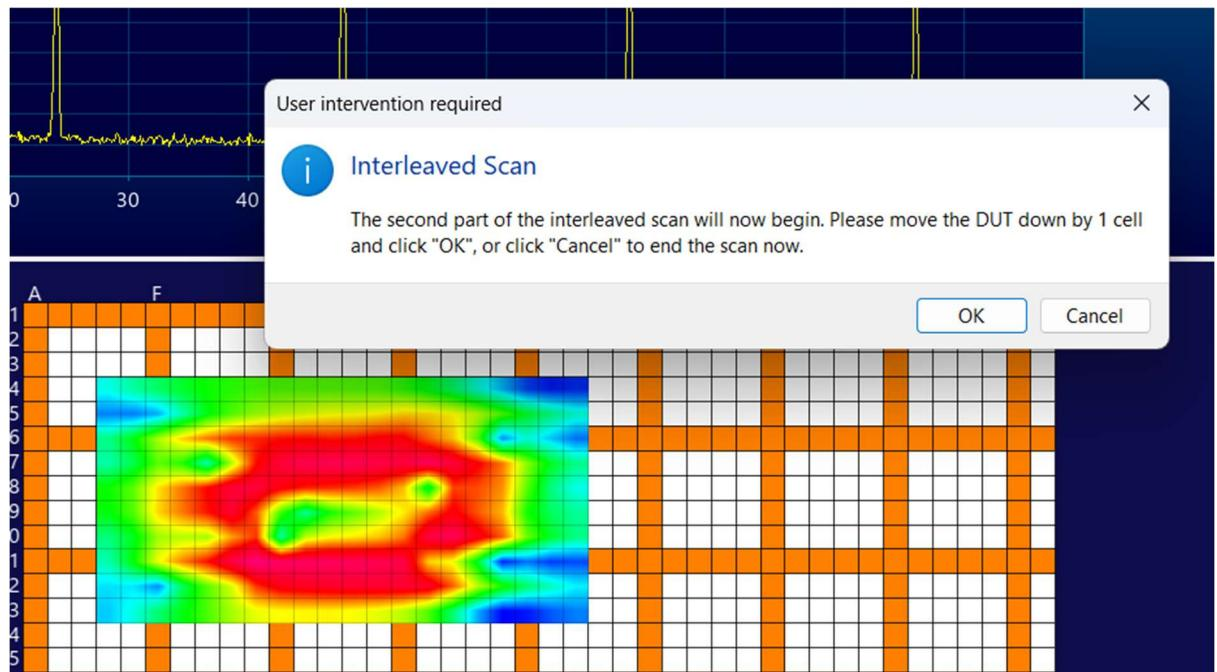
c. After the first scan, a message box will pop-up indicating to move the DUT down by exactly 1 row. Another way to describe the direction up is along the shorter axis towards the higher row numbers. Do not change the orientation or position along the longer axis of the board. After you move the DUT, click OK to run the second scan.
