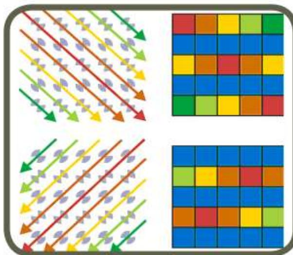
In certain situations, the presence of dead spots can create misleading results. An example of this is shown below. The image on the left shows a diagonal trace with one standard scan. The image on the right shows the same trace after two interleaved scans.
