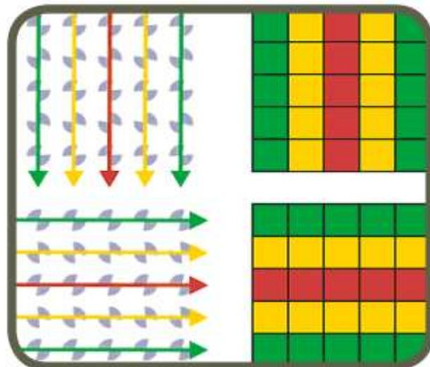
However, if the device has H-field components then every other row will have very low reception sensitivity. The scan results are shown below in the top right. Now if this device is rotated 90° then dead spots will switch to the alternate row. Although the high-level results are as expected, the presence of these low values distract the eye. Furthermore, since the dead spots do not rotate, they may give the impression that the scan results are completely different.
