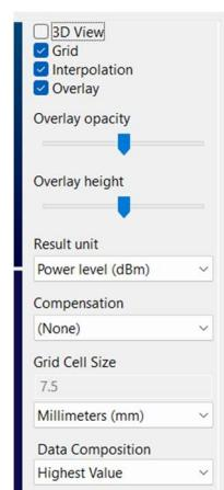
Grid and Overlay can be shown or hidden. Interpolation (data smoothing) can be disabled. You can also change the unit of amplitude or apply a compensation file.
