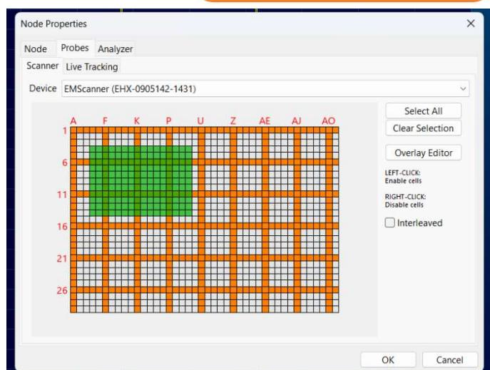
**Control level (EMSR only):** You can perform a high-resolution scan by increasing the control level. Each control level performs 4x the number of sweeps than the previous level. The resolution of the scan and how many measurements taken per cell is shown below the control level control.
